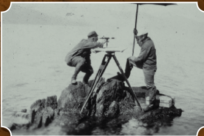
Coast and Geodetic Survey crew uses a plane table to map shoreline in Southeast Alaska circa 1921. Credit: NOAA.
